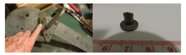
Trying to purchase a new rivet was difficult as nobody could supply, plus if I was to total dismantle the triangle I needed 3 rivets. They could be made and it would not have been the difficult, but I was told about a company in Brisbane called Power Window. This company only does window winders both electric and mechanical. They suggested having a look at my failed mechanism to see if they could supply rivets, with the idea of keeping the car as original as possible.
