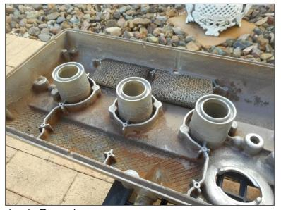
Interestingly, inside the cover there is an oil separator for the crankcase ventilation system. Jaguar in their wisdom made no provision for this plate to be removed in order to access and clean the two woven steel wool like pads underneath. What appears to be rivets holding the plate are, I suspect, dags cast on the bosses and then mushroomed over once the plate was in place. I removed the rivet like tops with my
