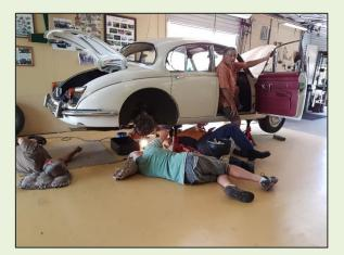
While the differential oil was being drained, the drive shaft was disconnected from it and then secured up under the car giving clearance for the next stage. The Drive flange bolts were 9/16 AF. Next was the removal of the drive flange. This needed a steel brace to stop it turning because the hand brake would not hold as the pinion shaft nut was being removed. The pinion nut is 1 1/8 AF. It put up a bit of a fight but with 11 determined amateurs it had no chance.
