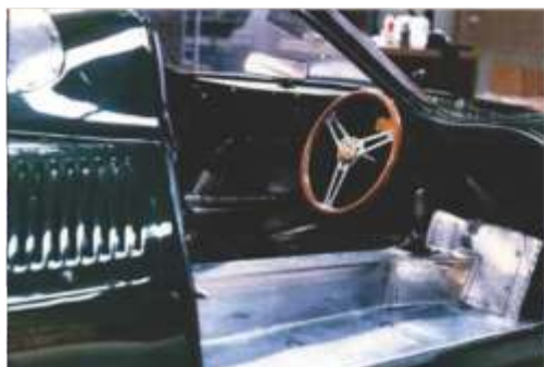
The inside of the XJ13 was pure racing car with bare aluminium, no insulation and aluminium radiator pipes running above the passenger floor.
