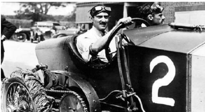
Note the shredded Tyre after a high speed run
